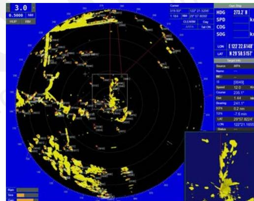
AIS and radar echo data can overlay display.
